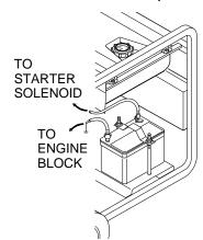
Figure 12 - Connecting Positive and Negative Cables to Battery (Model PGH11000IE Shown)
